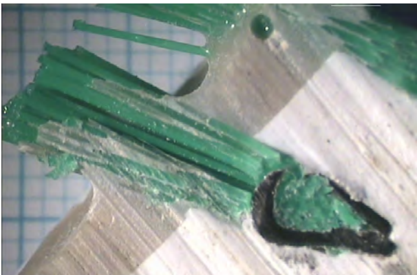
Courtesy of CampdenBRI. Channel, potential contamination trap in a resin set food industry
